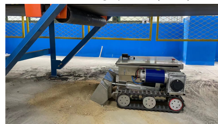
Fig. 1. An UTGV designed for cleaning purposes in mining.
