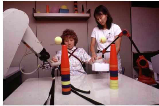
FIGURE 2.13: MIME workstation with PUMA-560 robotic arm in a therapeutic exercise [7].
